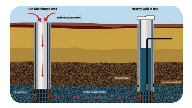
How surface water getting into old and abandoned water wells can contaminate water in wells being used for drinking water.
