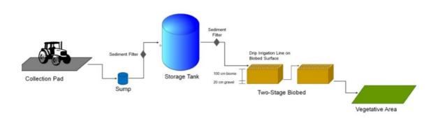
Schematic Diagram of a Two-Stage Bio-Bed
