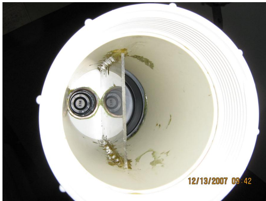
Figure 10. BENT Lab sample splitter from top view. Note the spigot outlet on the left, the dividing plexiglass in the middle, and the closed half chamber on the right (photo by I. Phillips).
