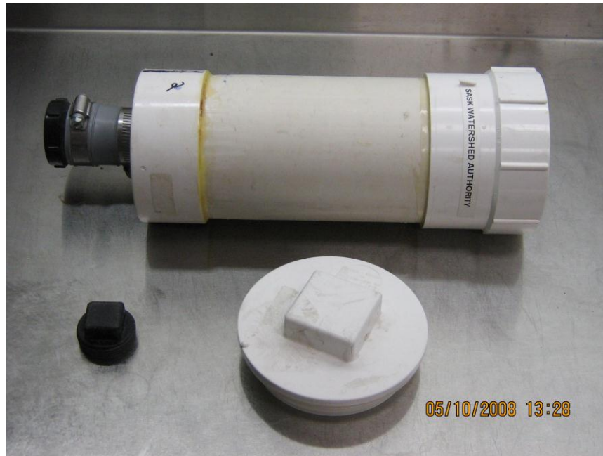
Figure 9. BENT Lab benthos sample splitter from side view with lid in the fore middle of the picture, and the spigot cap to the fore left in the picture (photo by I. Phillips).
